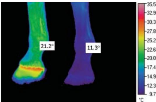
The camera can confirm whether there are heat anomalies in the leg or hoof, whether there is excessive heat possibly indicating an abscess, or cooler areas, often the symptoms of poor blood flow
